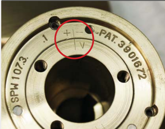
original factory pitch setting : markings line up
